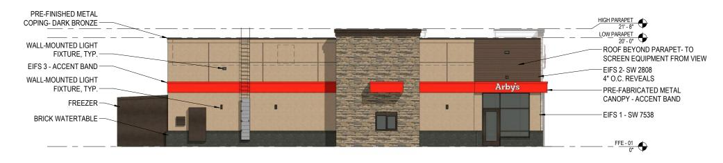
PROPOSED NORTH BUILDING ELEVATION SCALE: 1/8" = 1'-0"
